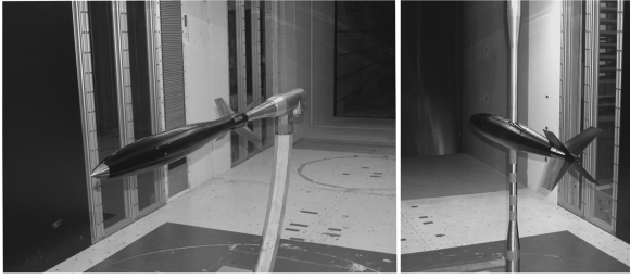
Fig. 1 Distorted MK-82 model and undistorted model with image supports.
